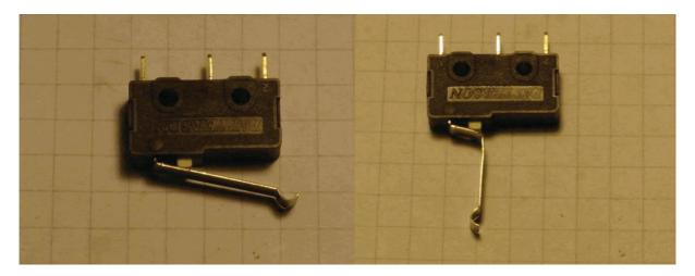
The switch is then epoxied to the base-board after checking, and adjusting if necessary, both the position of the switch and the amount of bend of the arm so that the switch closes when the piston is about half way between the limits of its travel.
