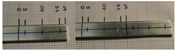
Step2: Drill the aluminium strip. The holes at each end of the finished section are 3mm, the one in the middle is 2.5mm. **Do not** be tempted to drill the middle one 3mm as well to save time. It is also important that the middle (2.5mm) hole is perpendicular to the strip. This is where a pillar drill will help if you have access to one. If doing it by hand, check the perpendicularity as carefully as you can.
