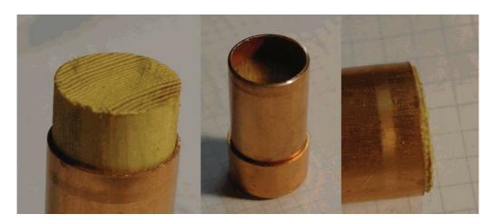
Step 6: Clean the inside of the stop end with steel wool. When all your piston parts are ready for assembly, mix the 2-part epoxy adhesive. I find that the 'quick setting' (15minute) variety is OK for this so long as you can complete all the pistons before the adhesive starts to gel.
