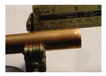
Step 2: Check that this piece of tube slides easily through a slip-coupling in all orientations. If it won't, or if it binds/rubs in places, cut a new length of tube.
