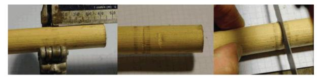
Step 4: 'Deburr' the inside of one end of the tube by filing away the turned-in edge left by the pipe cutter.
