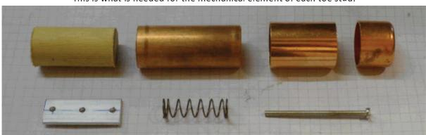
This is what is needed for the mechanical element of each toe stud:
