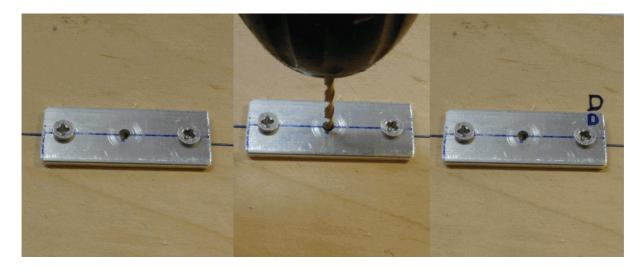
Step 6: Unscrew all the plates, turn the board over and bore 24mm holes using the 2.5mm holes to locate the borer. It is helpful to clamp the board to a solid work bench if possible, and place some scrap material below the board if you don't want holes in your workbench (or kitchen table!). Again, it is important to keep the hole perpendicular to the base board.
